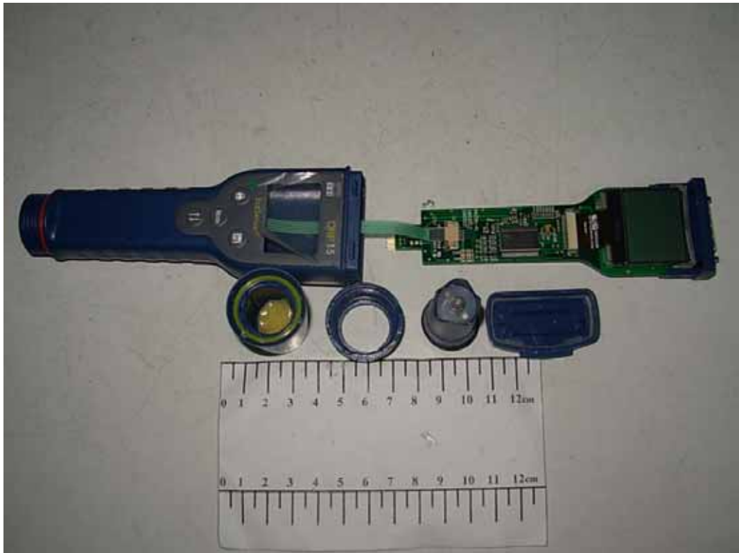
FIGURE 43 PH & TEMPERATURE/ORP & TEMPERATURE POCKET METER (M/N: ORP15N) COVER REMOVED
