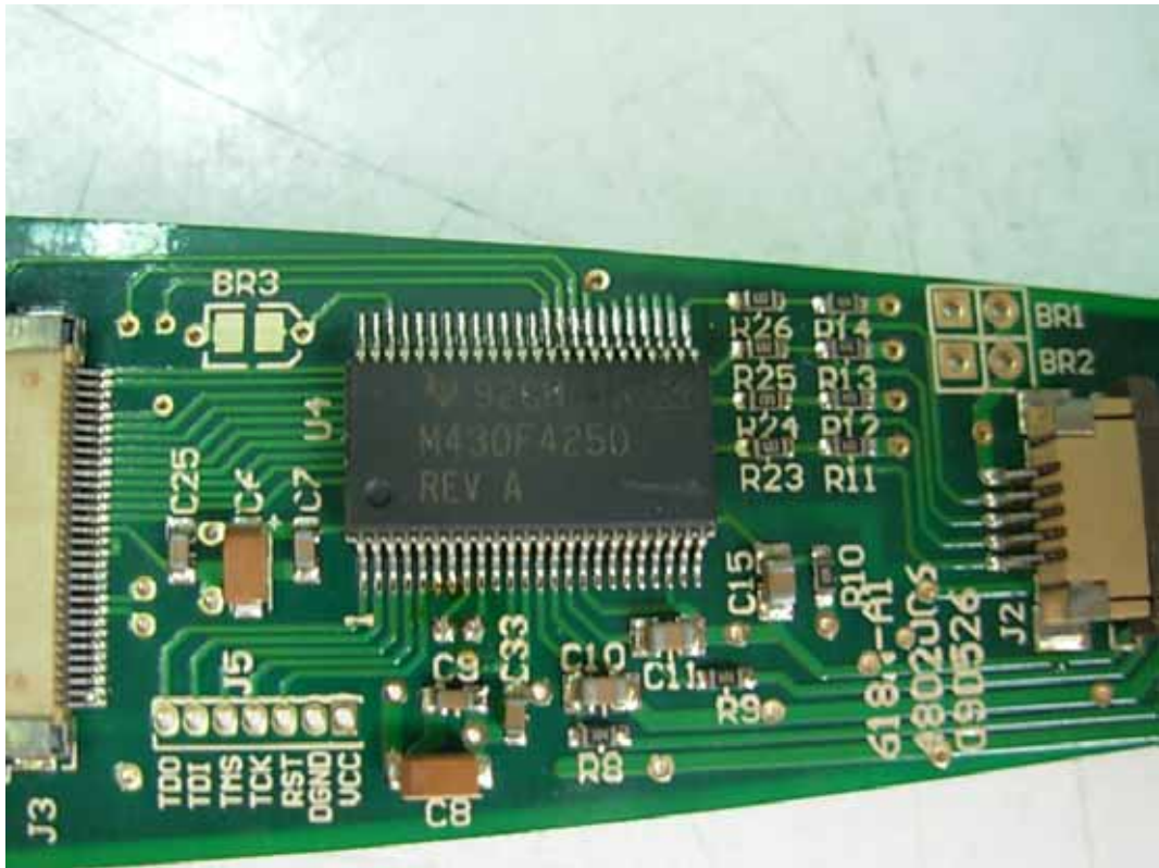
FIGURE 16 PH & TEMPERATURE/ORP & TEMPERATURE POCKET METER (M/N: 619) CHIP ON MAIN BOARD
