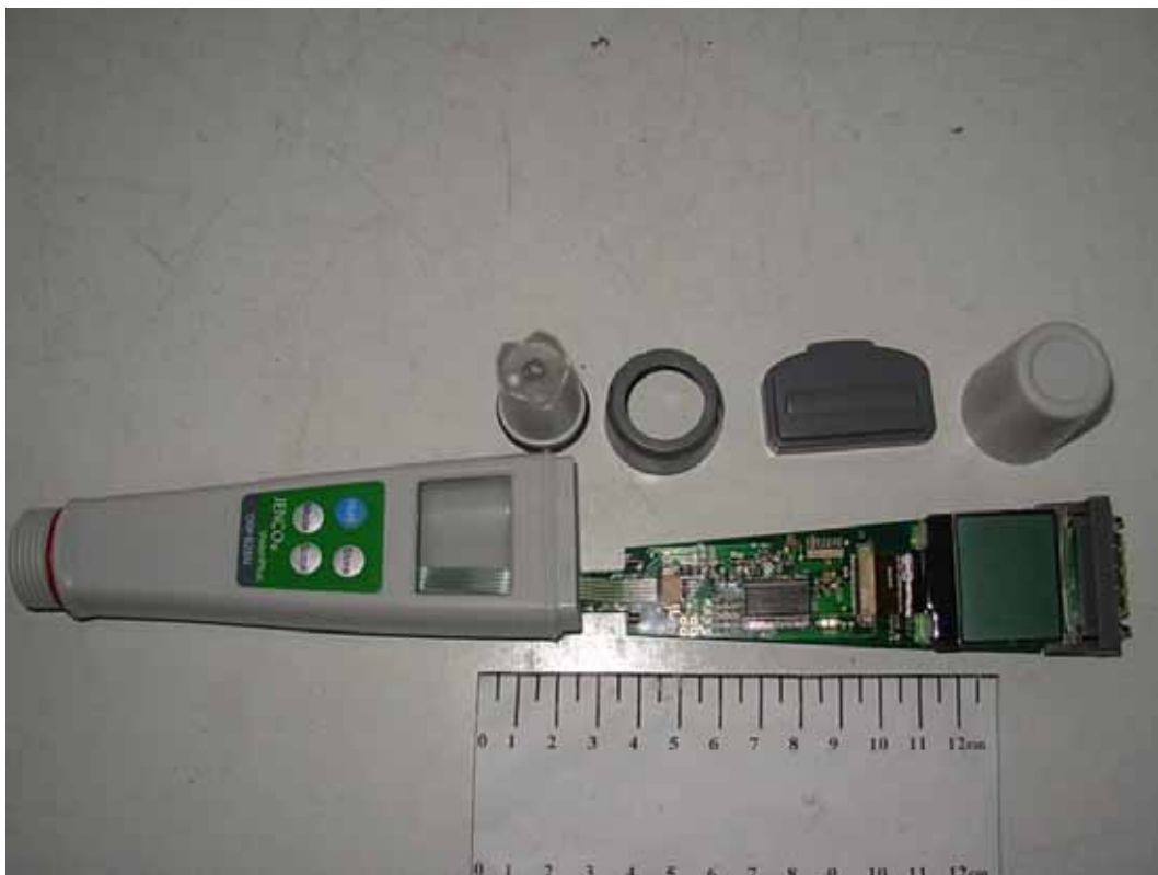
FIGURE 36 PH & TEMPERATURE/ORP & TEMPERATURE POCKET METER (M/N: 628N) COVER REMOVED
