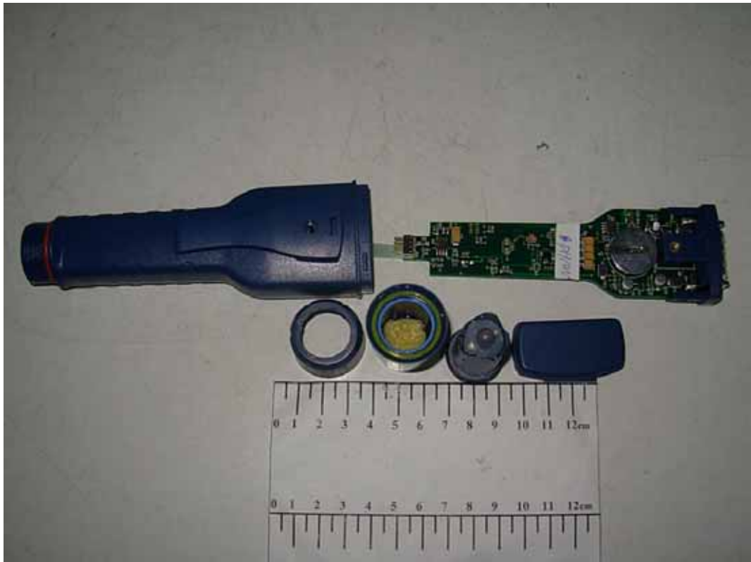
FIGURE 28 pH & TEMPERATURE/ORP & TEMPERATURE POCKET METER (M/N: PH10N) COVER REMOVED
