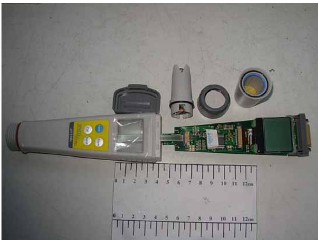
FIGURE 4 pH & TEMPERATURE/ORP & TEMPERATURE POCKET METER (M/N: 618N) COVER REMOVED
