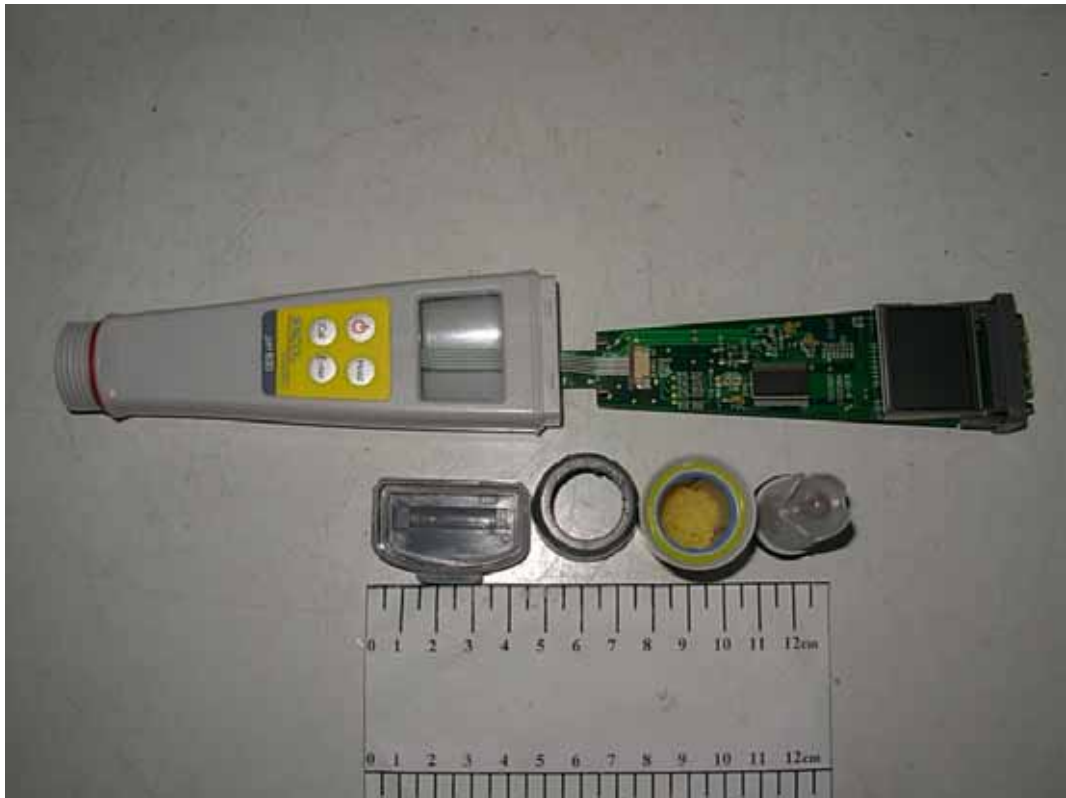
FIGURE 20 pH & TEMPERATURE/ORP & TEMPERATURE POCKET METER (M/N: 630) COVER REMOVED
