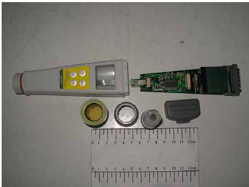
FIGURE 12 pH & TEMPERATURE/ORP & TEMPERATURE POCKET METER (M/N: 619) COVER REMOVED
